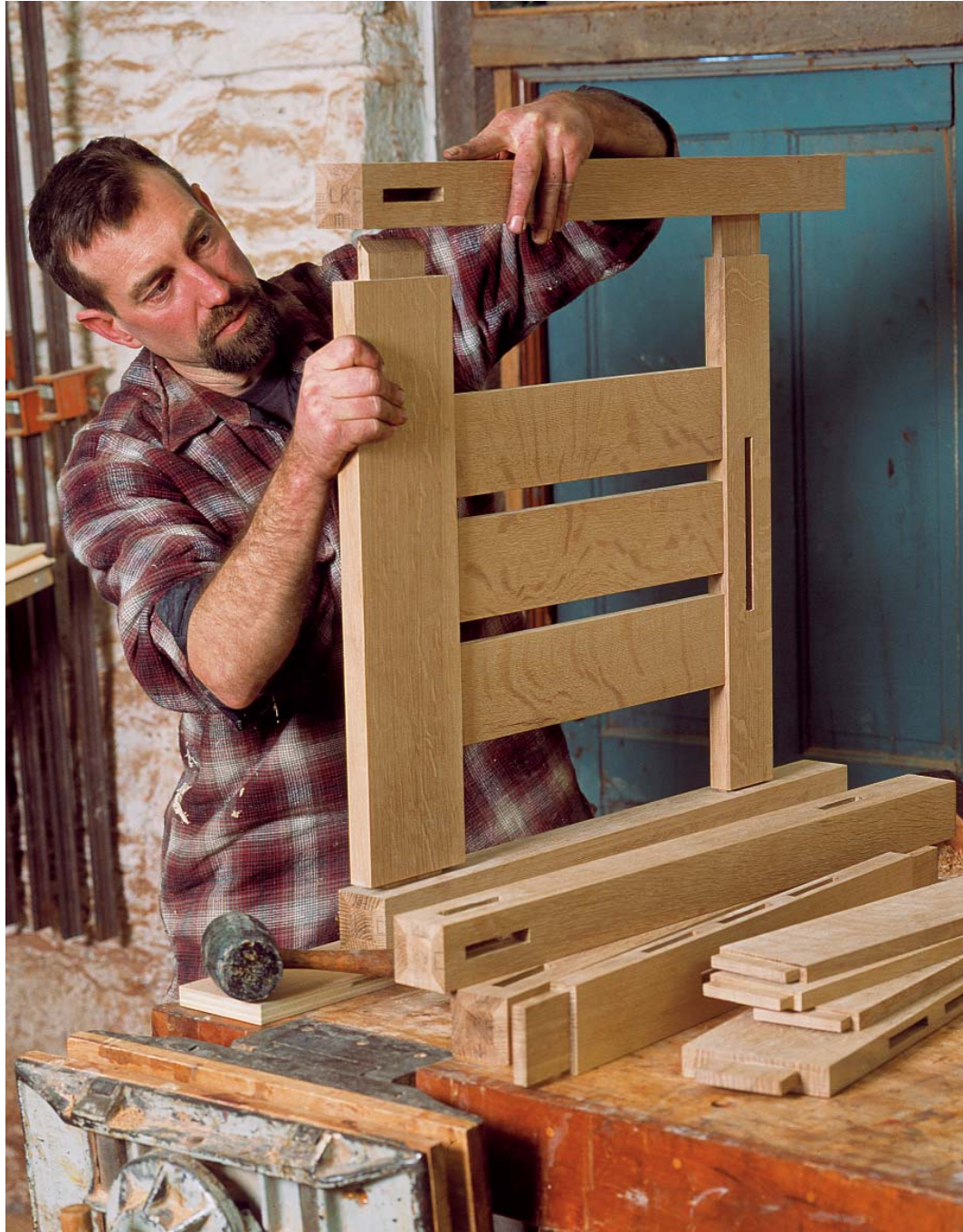
Assemble the ends. First fit the slats to the apron and lower rail, then set the assembly into the mortises on the legs.
