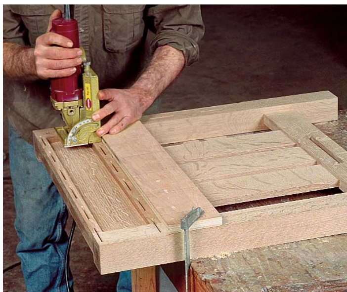
Assemble the ends. First fit the slats to the apron and lower rail, then set the assembly into the mortises on the legs.
