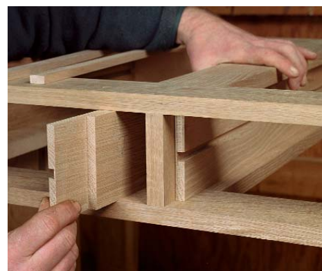
Glides span the dividers. Center dividers are sandwiched between two filler boards that house the drawer glides.
