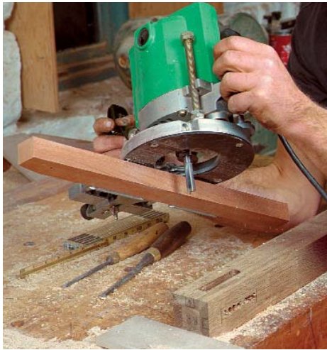
Route the mortises. Using an edge guide on a plunge router, drop the bit a little at a time until you reach the desired depth.
